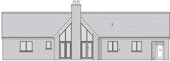
PROPOSED SOUTH EAST ELEVATION Scale 1:100 1. Facing brickwork 2. uPVC Windows/Doors 3. Tiled roof 4. Recessed Porch
