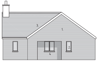
PROPOSED NORTH EAST ELEVATION Scale 1:100 1. Facing brickwork 2. uPVC Windows/Doors 3. Tiled roof 4. Recessed porch
